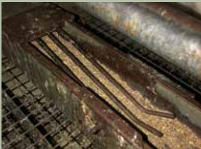
Chick saver in aviary rearing to prevent that DOC moving in the running feed chain
