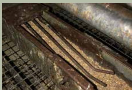
Chick saver in aviary rearing to prevent that day old chick moving in the running feed chain
