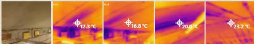
A good transverse ventilation system is intended to warm up the incoming air by directing it to the roof where the air temperature is higher. This sequence of thermal images you can see the effect of an optimal transverse ventilation
